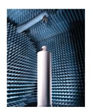
ETS-Lindgren's AMS-8800 Series Antenna Measurement System is a theta arm based antenna measurement test system. This system is ideally suited for automated measurement of antenna performance of wireless devices and devices with embedded wireless functions. The AMS-8800 includes a distributed axis positioning system consisting of an azimuth rotator to rotate the AUT about the phi axis and a separate theta arm positioner to elevate the measurement antenna around the AUT.
